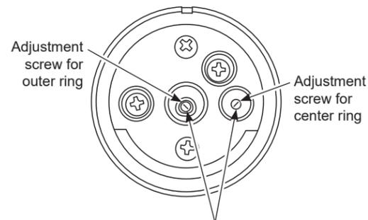
Adjustment screws for multi-ring burner only
