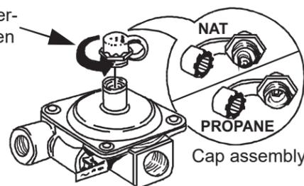
3. Turn the metal cap so the type of gas being converted to is displayed and replace the protective plastic cover.
